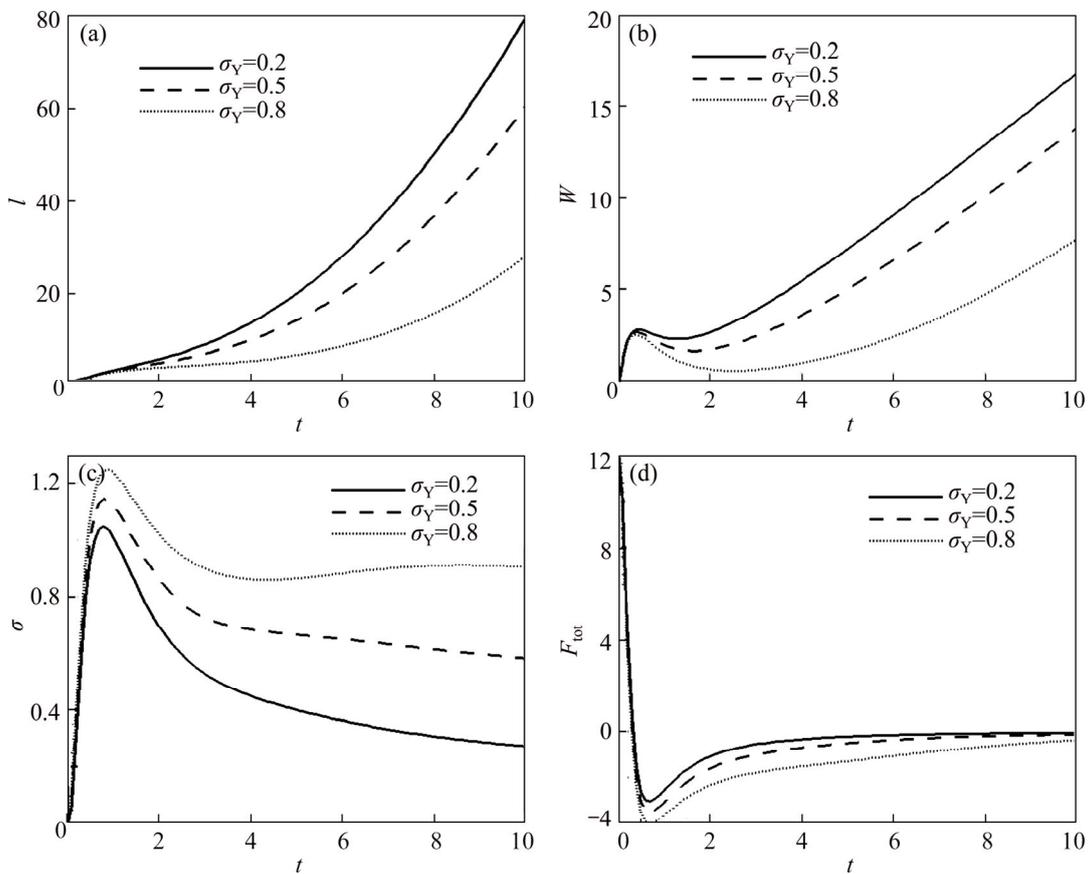
**Fig. 3** Elongation (a), velocity (b), stress (c) and total force (d) as a function of time for different values of  $\sigma_Y$  when  $n=1.8$
