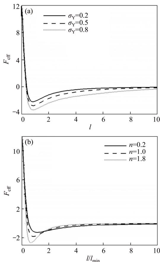
**Fig. 4** Effective forces as a function of elongation= $l$  for different values of  $n=1$  (a) and  $\sigma_Y=0$  (b)
