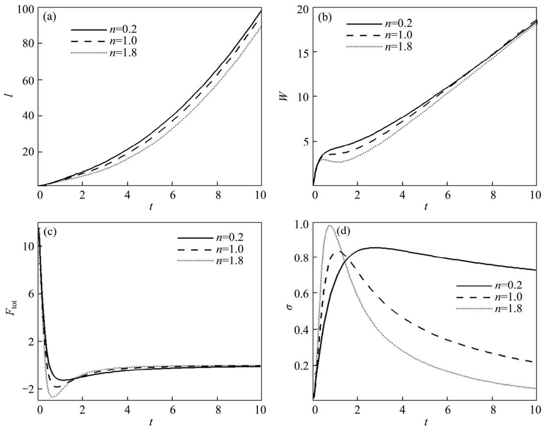
**Fig. 2** Elongation (a), velocity (b), total force (c) and stress (d) as a function of time for different values of  $n$  when  $\sigma_Y=0$
