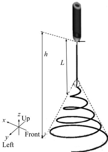
Fig. 1 Schematic drawing of electrospinning process
