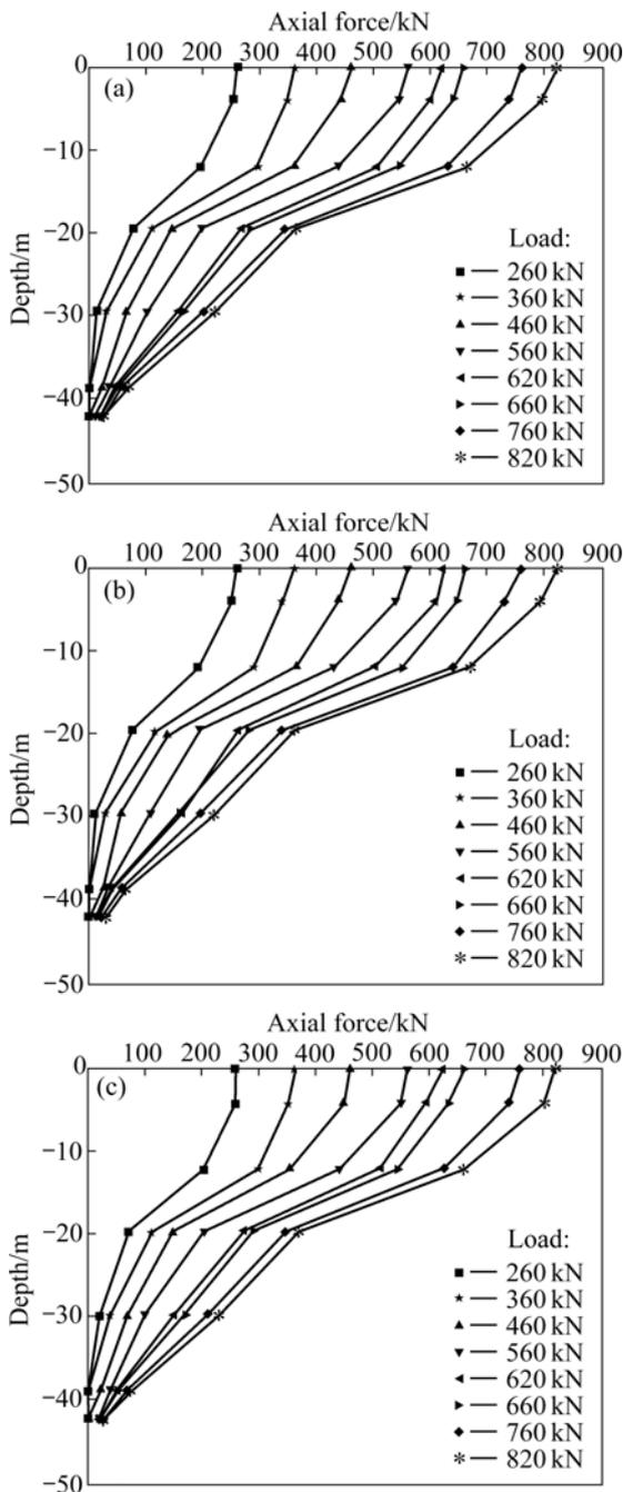
**Fig.4** Axial load transfer curves for piles 1–3: (a) Axial force distribution for pile 1; (b) Axial force distribution for pile 2; (c) Axial force distribution for pile 3
