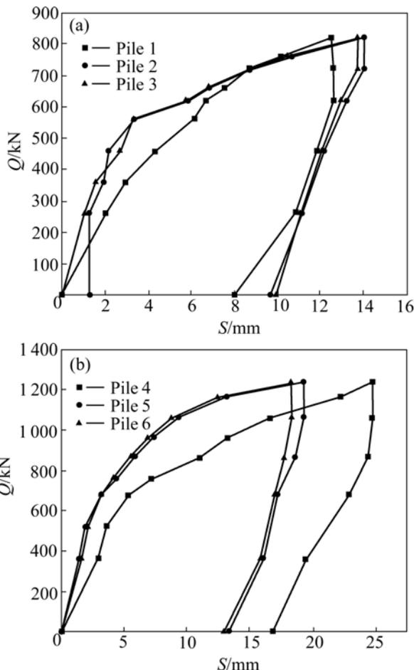
Fig.3 Static load test curves for different piles: (a) Piles 1–3; (b) Piles 4–6
