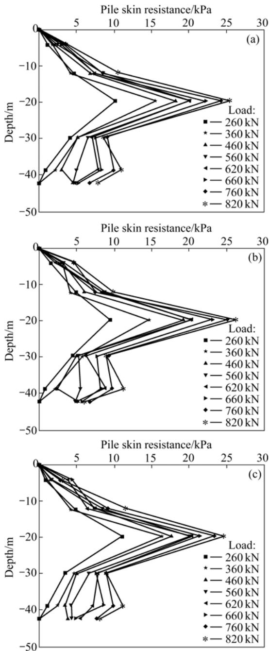
Fig.6 Pile skin resistance distribution for different piles: (a) Pile 1; (b) Pile 2; (c) Pile 3
