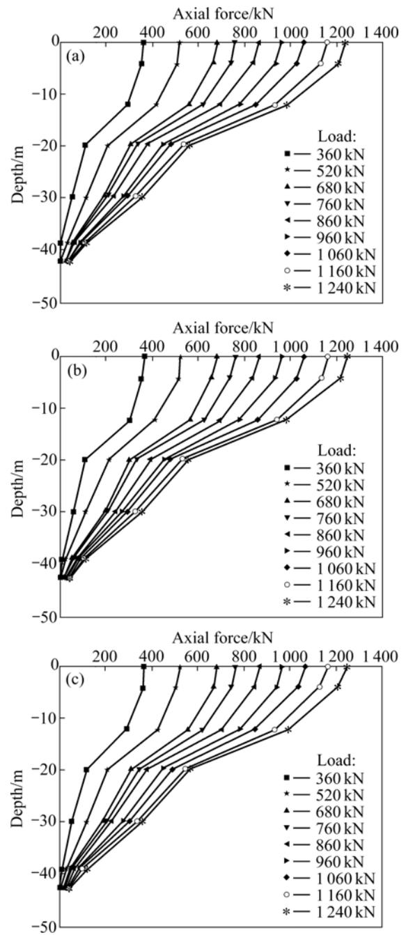
**Fig.5** Axial load transfer curves for piles 4–6: (a) Axial force distribution for pile 4; (b) Axial force distribution for pile 5; (c) Axial force distribution for pile 6
