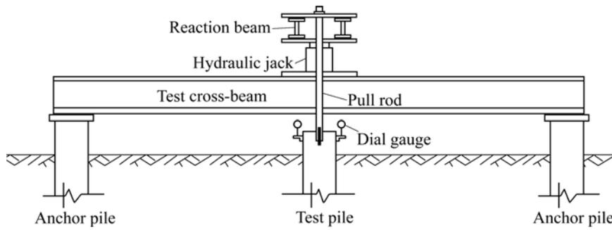
Fig.2 Pullout load test setup
