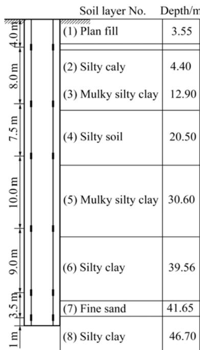
**Fig.1** Position of steel stress gauges
