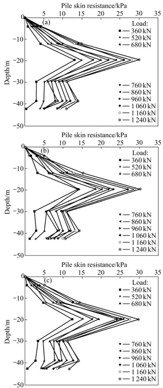
Fig.7 Pile skin resistance distribution for different piles: (a) Pile 4; (b) Pile 5; (c) Pile 6
