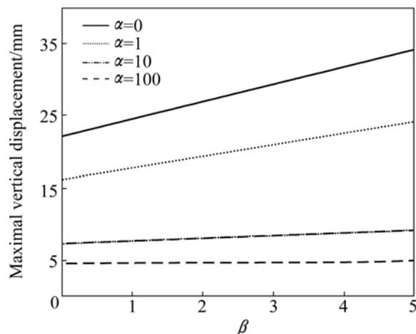
**Fig.7** Effects of temperature gradient coefficient  $\beta$  on maximal vertical displacement at different rotational stiffness of joints
