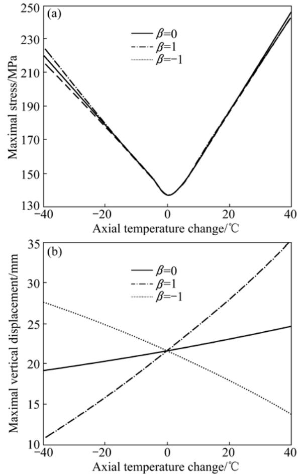
Fig.5 Effects of temperature actions on elastic behavior of steel beams: (a) Maximal stress; (b) Maximal vertical displacement
