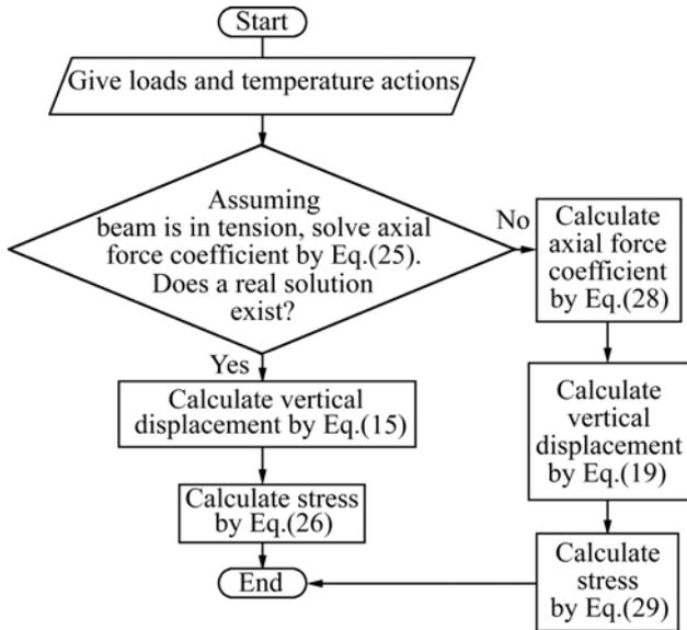
Fig.3 Flowchart for analysis of numerical example
