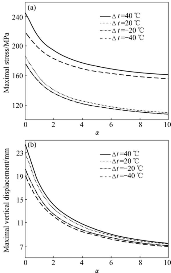
**Fig.6** Effects of rotational stiffness of joints: (a) Maximal stress; (b) Maximal vertical displacement
