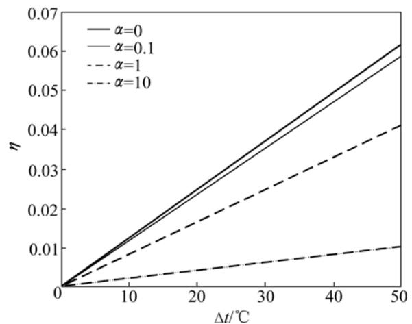
Fig.2 Effect of temperature gradient (Δt) on axial force coefficient (η)
