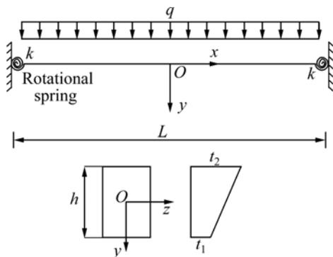
Fig.1 Geometric model of steel beams
