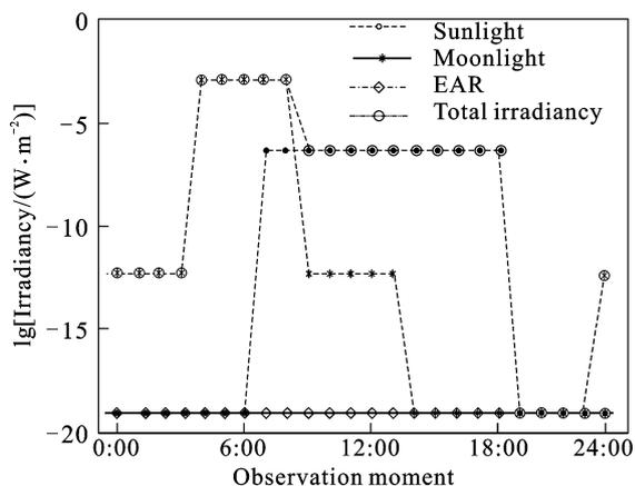
**Fig. 10** Space luminous environment of star sensor on September 20, 2011
