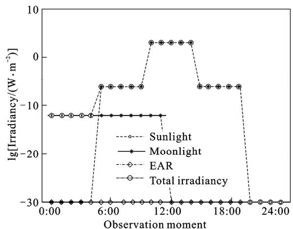
Fig. 9 Space luminous environment of star sensor on Summer Solstice
