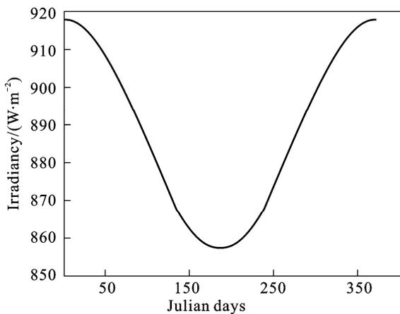
**Fig. 1** Sun irradiancy at star sensor working height in star sensor spectral range
