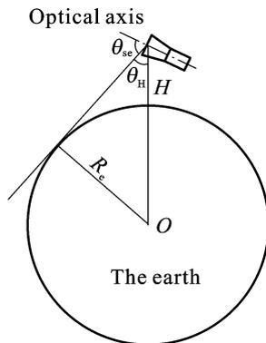
Fig. 3 Schematic diagram of EAR and star sensor optical axis
