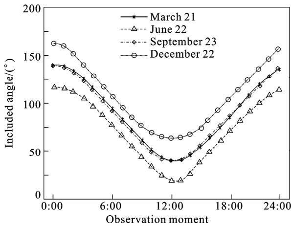
Fig. 7 Included angle between star sensor optical axis point and sunlight
