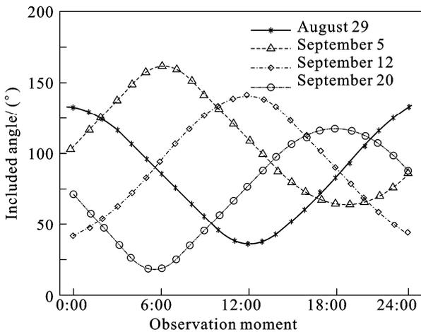
Fig. 8 Included angle between star sensor optical axis point and moonlight
