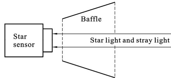
Fig. 4 Installation positions of star sensor and baffle
