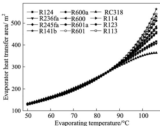
**Fig. 6** Evaporator heat transfer area versus evaporating temperature for ORC with IHE but without PHE
