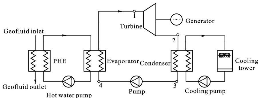
Fig. 1 Schematic diagram of actual ORC geothermal power plant
