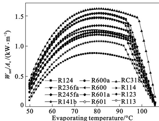
**Fig. 8** Ratio of net power output to evaporator heat transfer area versus evaporating temperature for ORC with IHE but without PHE
