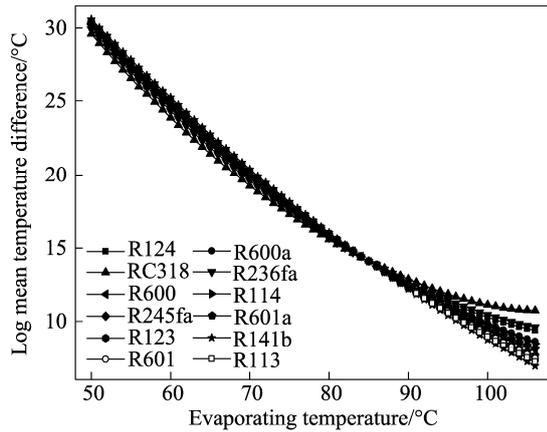
**Fig. 5** LMTD versus evaporating temperature for ORC with IHE but without PHE
