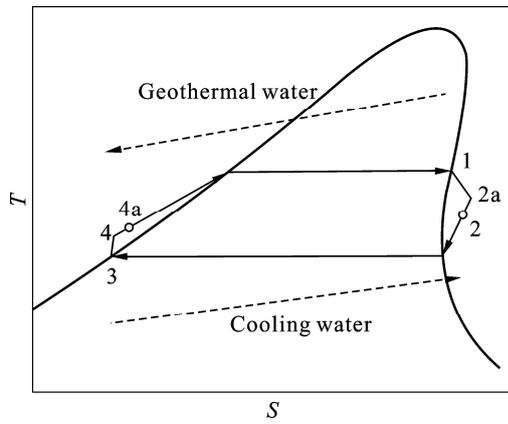
Fig. 3 T-S diagram of modified ORC
