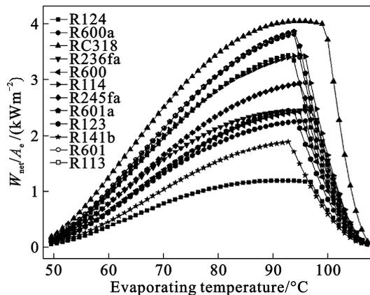
**Fig. 9** Objective function versus evaporating temperature for ORC with IHE but without PHE
