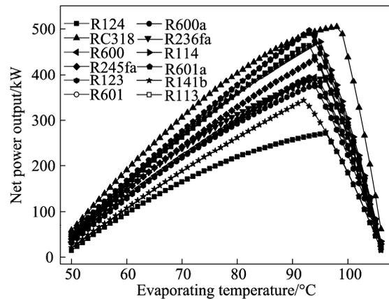
**Fig. 7** Net power output versus evaporating temperature for ORC with IHE but without PHE
