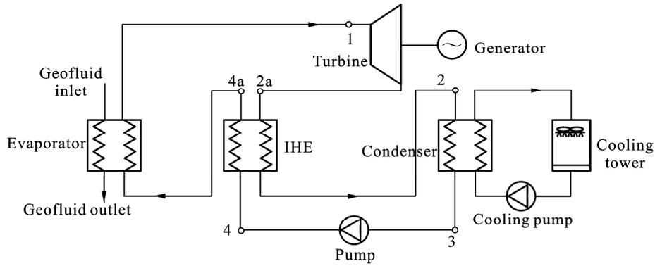
Fig. 2 Schematic diagram of modified ORC geothermal power plant
